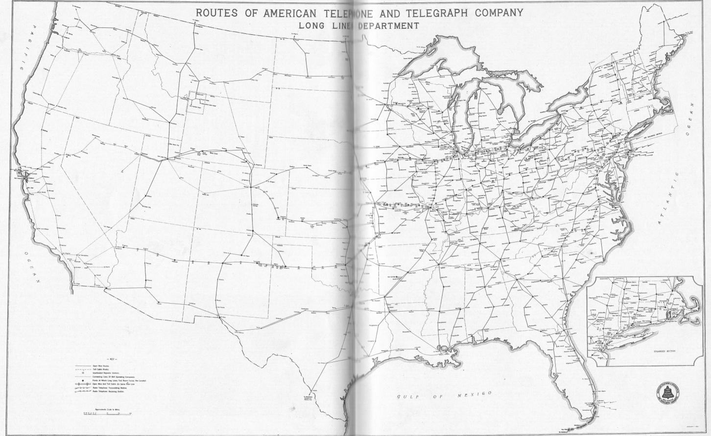
Figure 30. Open wire and cable lines of the Long Lines Department.
